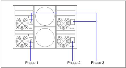
Figure 71: Single basic unit with a 3-phase input
